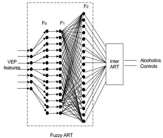
Fig. 3 SFA network as used in the study
