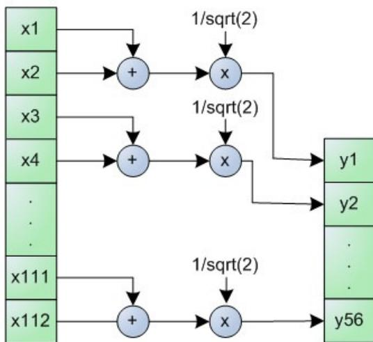
Figure 7. First level of wavelet decomposition
