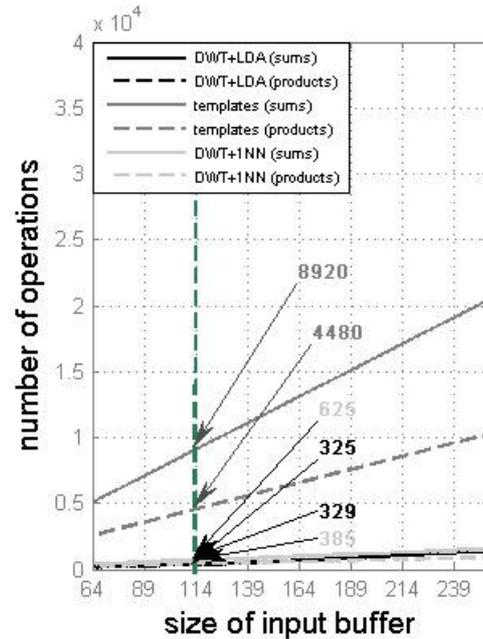
**Figure 4. Number of operations versus buffer size for the vertical channel having four classes**
