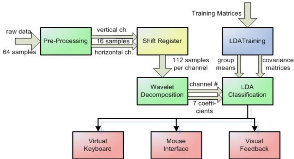
Figure 6. Flow diagram of the EOG interface
