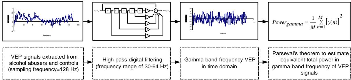
Figure 3: Procedures involved in the proposed method (Method A)
