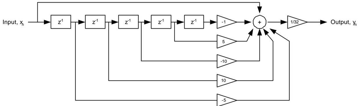
Figure 1: Realization of the proposed high-pass digital filter to extract gamma band VEP
