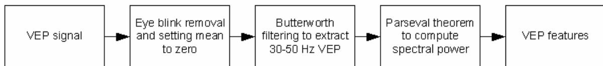
Figure 5: Steps in the feature extraction process
