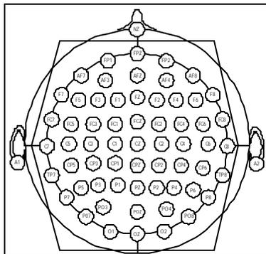
Figure 1: Locations of electrodes (61 active channels inside hexagon)
