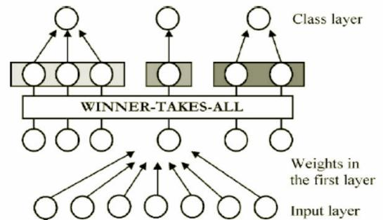
Figure 4: Structure of GAL Network
